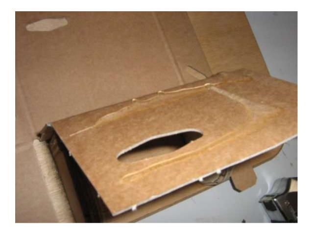
Phase 5; lift the corner piece and apply two lines of glue.
