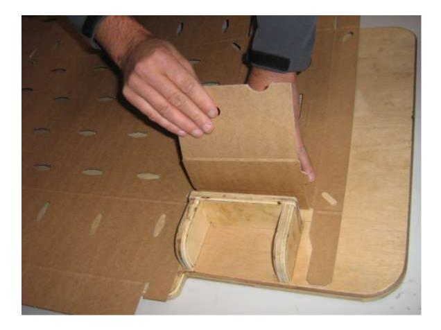
Phase 2; push the die cut down and fold the corner pieces up.
