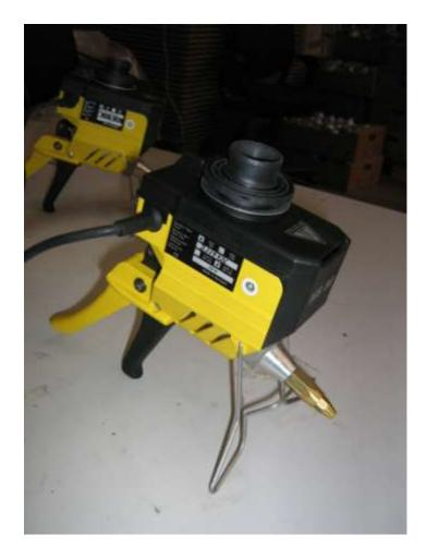
Disconnect the hotmelt gun from the power supply.
