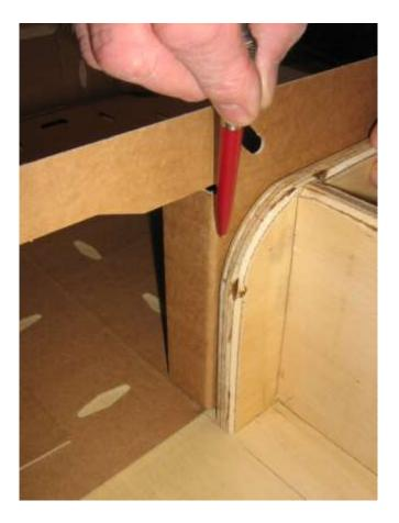
Phase 4; make sure the die cut is positioned exactly in between the supports on the frame.
