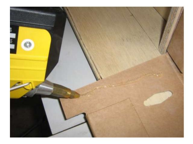
Phase 7; Apply one line of glue along the whole length. Apply glue on the left and on the right corner.
