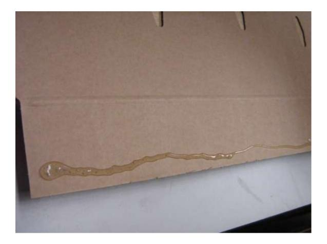
Phase 2; make sure there is sufficient glue on the corners of the flaps.
