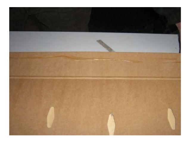
Phase 2; apply glue along the outer edge of the flap.
